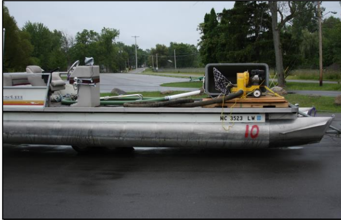
Figure 30. A DASH boat for hand-removal of milfoil or other nuisance vegetation. ©Restorative Lake Sciences, LLC
