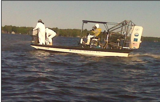
Figure 28. An airboat used to apply aquatic herbicides.
