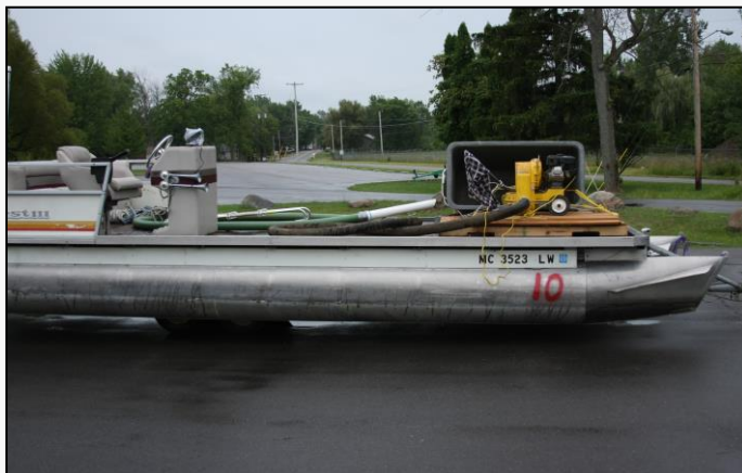
Figure 44. A DASH boat for hand-removal of milfoil or other nuisance vegetation. ©RLS
